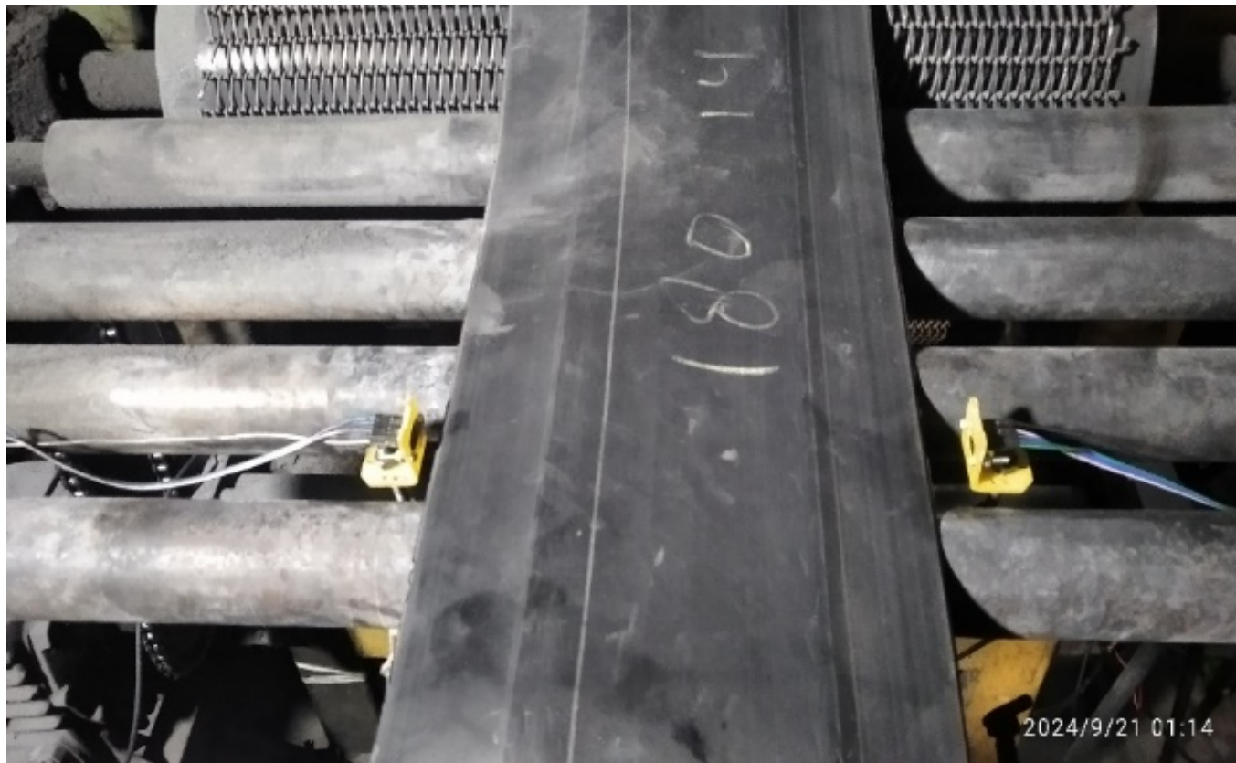
Figure 10. Pengujian Sensor VL53L0X
