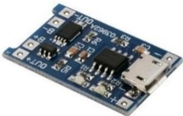
Figure 5. Modul Charger TP-4056
