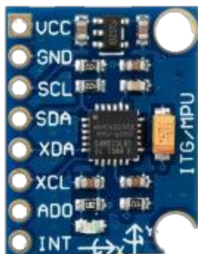
Figure 4. Sensor Akselerometer MPU-6050
