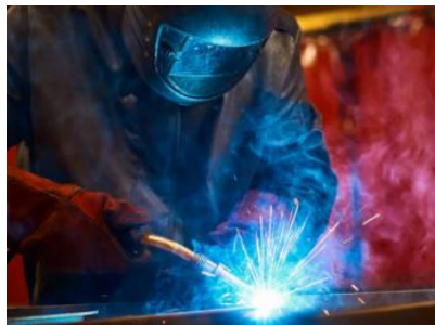
Gambar 4. Proses Pengelasan Metal Inert Gas (MIG)
