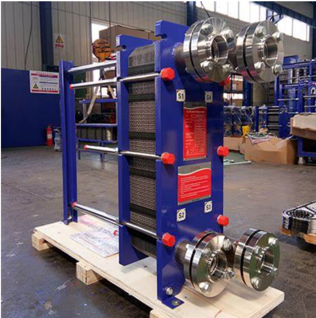
Figure 2. Gambar 2. Heat exchanger dan plat Heat Exchanger
