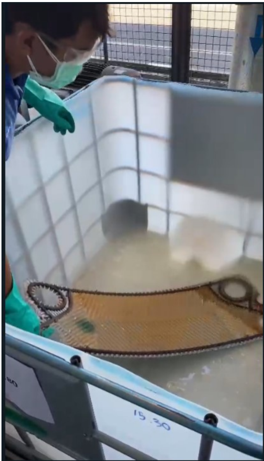
Figure 4. Heat exchanger dan plat Heat Exchanger Gambar 3. Proses Perendaman Plat And Gasket Heat Exchanger
