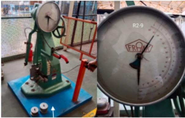
**Figure 16.** *Alat Uji impak Metode Charpy*
