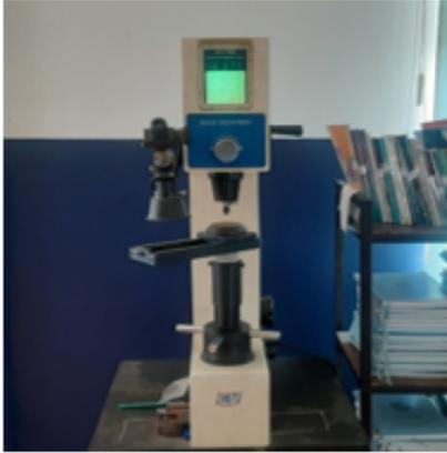
**Figure 20.** *Alat Uji Kekerasan*
