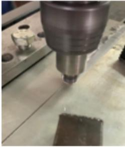
**Figure 14.** *Proses Pengelasan FSW*
