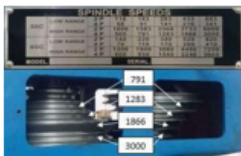
Figure 10. Setting Kecepatan Putaran Spindle
