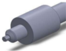
Figure 1. Desain tool FSW Geometri Hexagonal
